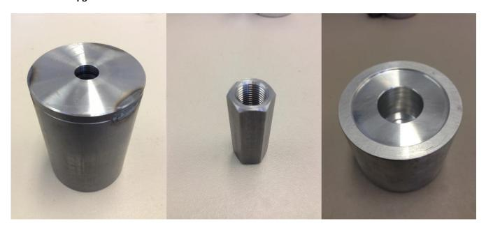
Top row, left to right: MY06-08 bearing puller housing (left). Replaces puller tube from IMS Pro-Tool kit when pulling bearing. Use with 06-08 Hex adapter (center) to thread onto center stud. 06-08 driver tool shown for installing new bearing (right). Use a dab of grease to help hold bearing to driver if desired.
