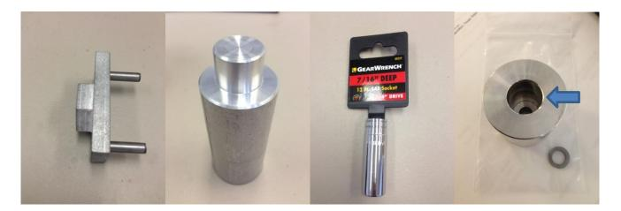
Bottom row, left to right: IMS Solution spin on filter adapter spanner tool (left). IMS Solution oil plug installation tool ( $2^{ND}$  from left). Use a dab of grease to help hold plug (included in IMS Solution kit) to driver if desired. Narrow 12 pt socket for torqueing center nut on IMS Solution ( $3^{rd}$  from left). Bushing/bearing driver spacer insert – goes into the counterbore of the Pro Toolkit's bearing driver to accommodate for the longer center stud in the IMS Solution.
